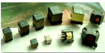
XDSL Transformers/POTS Inductors
